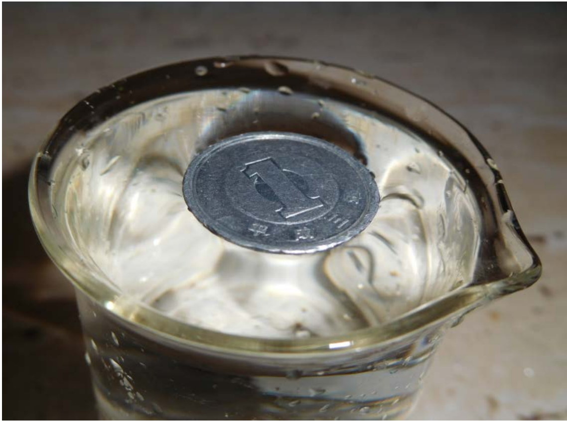
Figure 1: Camera capture of a running experiment and measurement coin floating on the water surface. The floating coin is well identifiable; however, this shot does not provide enough information for a measurement.
